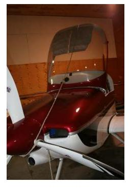
If your canopy rail has not yet been drilled, consider drilling the holes in the rail a bit lower than Van's instructions. Drilling per Van's, puts the top edge of the mount above the edge of the canopy deck. It will look nicer lowering the mount holes. You do however have to make sure the gas cylinder has adequate clearance to the canopy deck.
