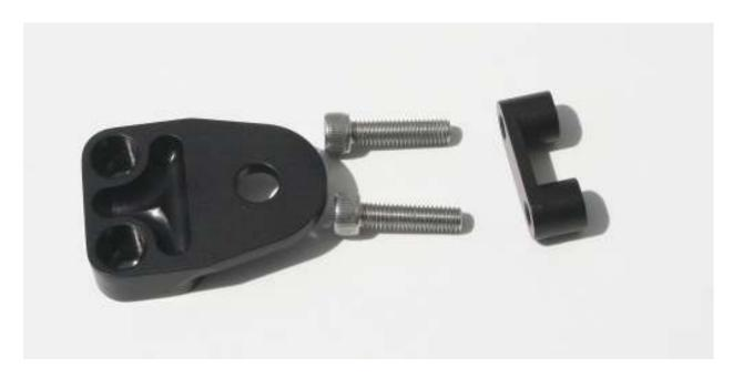
We start with a billet knob mount. This beauty is anodized for looks and protection. One of the biggest advantages is the nut assemblies. They are linked together so that no tools are required in the limited space behind the canopy deck. The dip in the middle of the nut assembly allows room for a fingertip to push the flat side of the nut up to the aircraft structure.
