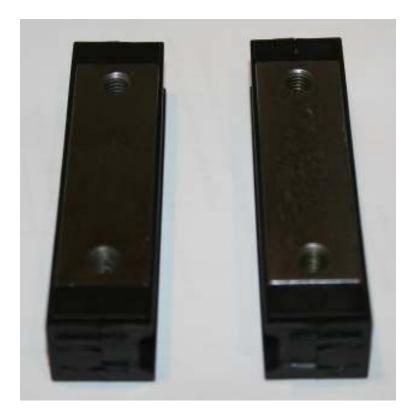
Remove the 4 screws noted as fixed and adjustable bearing attachment screws. These are low head screws, so make sure you clean out any debris or corrosion in the socket area. Use a sharp 5mm allen wrench, engage it fully and squarely. Remove both individual bearings of the bearing pair. Clean the aluminum carriage with scotch brite. Note that there is a lip on the fixed edge of the carriage block.
