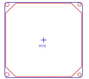
Select the chamfer command. It first asks you to specify the chamfer distance. Enter 0. Select the chamfer command and select the top line and the top left diagonal line to trim the ends. Repeat with the other lines until we have the octagonal ATI shape.
