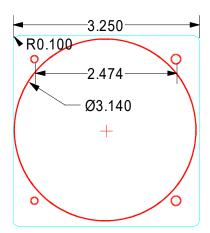
Consider the instrument to the left as a manufacturer may draw it. This is a standard cutout for a 3.125" instrument with allowance for paint.
