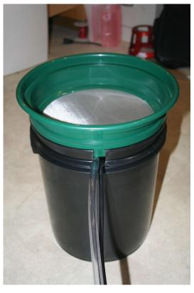
Connect the 3/8 ID tubing from the coolant pump to the elbow near Y axis stepper motor
