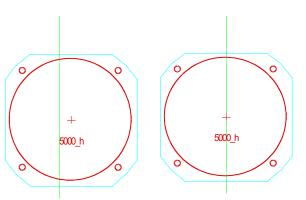
(intersection). Click on the vertical line, then click on the horizontal line that comprises the center mark of the instrument. The instrument will move from the center of the instrument to the intersection of the vertical line and the horizontal line of the center mark.
