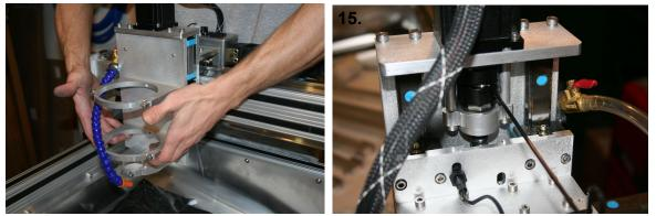
Install the Z axis motor with the 4
