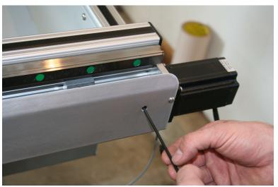
Access to the coupler clamp screw is through a hole in the lead screw guard. **Make** sure there is no slippage between the coupler and lead screw.
