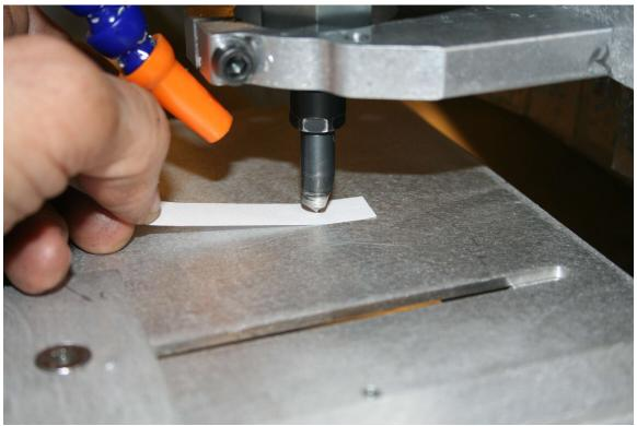
The tool installed in the picture is a 100 degree countersink. It can be used for countersinking and chamfering.
