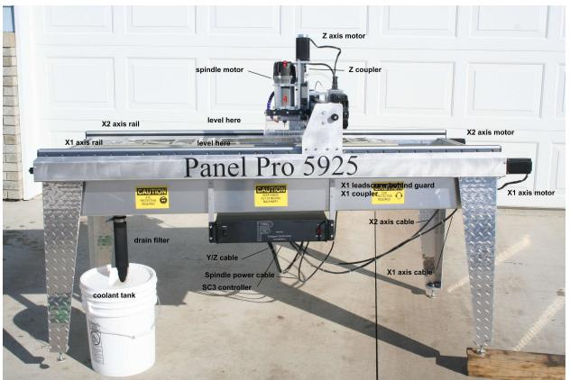
The purpose of the Panel Pro is to route complex assemblies of lines, points, circles, and arcs in sheet aluminum. It accomplishes this by reading a dxf file generated by popular computer aided drafting programs. This is especially useful since commonly used shapes such as instrument cutouts can be drawn and stored for subsequent combination into various instrument panels. The machine is also useful to fabricate various adapters and brackets that have many corners and cutouts.
