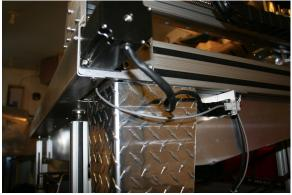
**21.** Locate the nuts with screws installed on the bottom of the right rail. Allow enough room to comfortably attach the motor plug. X2 axis is shown.
