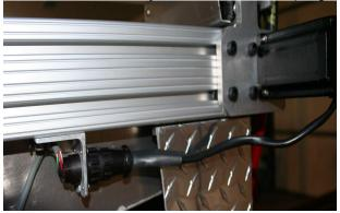
**22.** Attach the Y/Z cable and route cable. The Y/Z cable is the same on both ends and it does not matter which end goes on the controller or the Y axis. Note in the picture the X2 axis lead screw guard is not installed and the spindle (router) power cord should run parallel with the Y/Z cord.
