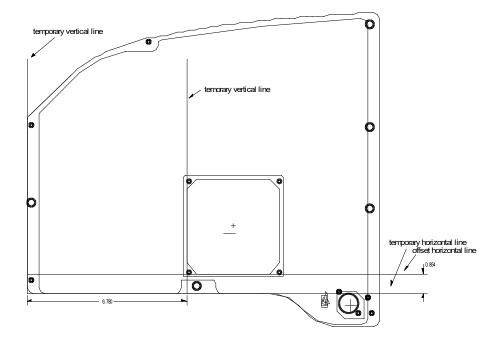
You can now draw a construction line from the center of the instrument and then draw offsets from that to place other instruments on the same vertical or horizontal centerline. If you have two intersecting lines you can place an inserted instrument (instruments have there 0,0 point in the center) by clicking mod>intersection or F6, then clicking on the intersection of the two lines you want to place it on.
