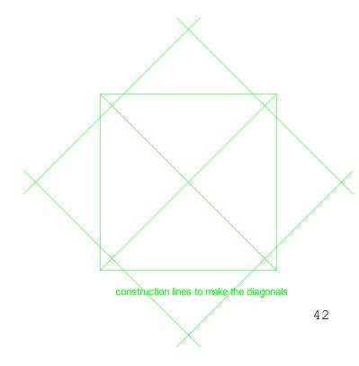
Draw a line from the lower right corner using object snaps (end point) diagonally to the left top corner, also using the end point snap to precisely locate the end point.
