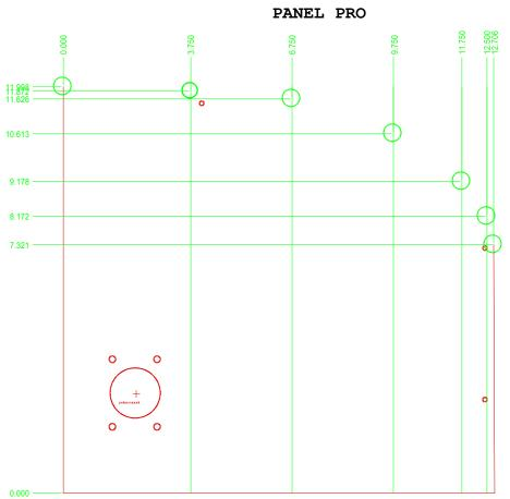
Now we will connect these points using the center snap (F4) with a parabolic spline. AvCAM does not support parabolic splines, however, when exported to a dxf file, EasyCAD breaks it down into a normal polyline with a bunch of segments.
