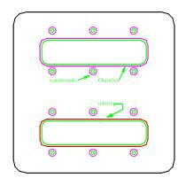
In this picture, the green entities were cut through, the red line on the bottom cutout defined the inlet, the purple entities were on a countersink layer and defined the countersinks and chamfers.
