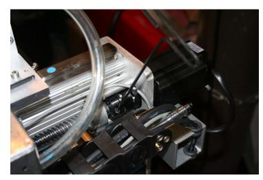
**13.** Install the "Y" motor in a similar fashion. Attach the Y motor to the connector closest to the motor. Tighten coupler to lead screw. Make sure it does not slip.
