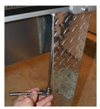
When leveling is as close as you can get it, adjust the leg glides on the left end so that both x1 and x2 lead screws touch their stops simultaneously.
