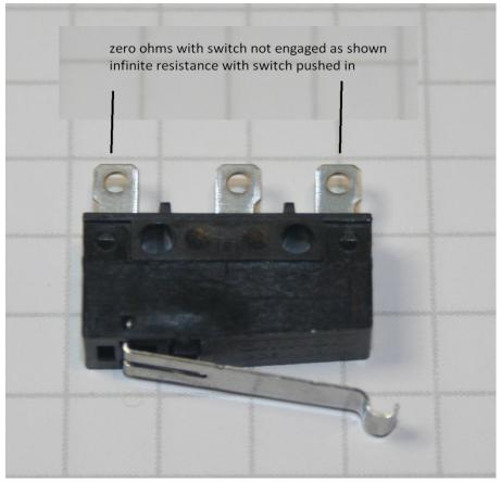
If the circuit is shorted or the switch has low resistance when opened, or the switch has been adjusted too close to the motor end, axis will hit the hard stop and chatter until the power is turned off to the controller or the pause switch is set to pause (early 5925s did not have a pause switch on the controller). The ESC key will not stop the movement in a home procedure.
