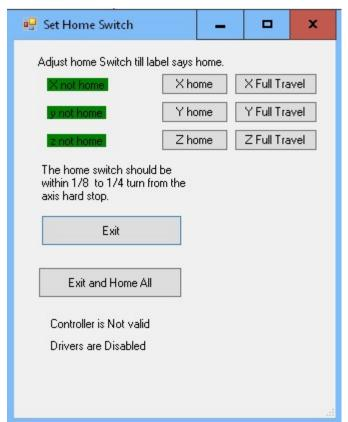
The hard stop on a X axis consists of a set screw in both X axis motor plates that will make contact with the Y axis end plate (the one with the knob on the Y axis ball screw) and the Y axis motor plate (the one with the Y axis motor mounted to it). When properly adjusted, the X axis home should be within .062" from the hard stop.
