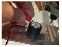
To set z zero, make sure the clip is attached to the end mill and the touch pad is directly below the end mill. Click "Probe End Mill".
