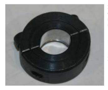
Install snap ring repair clamp pn 7-0100-0 with the lip in the existing snap ring groove. Use of red Loctite on the mating surface is recommended. Do not get Loctite on the mating surface under the bearing.
