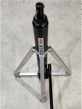
Carefully read and comply with the safety information of the Harbor freight Jack. While the maximum extended height is 45 inches, only raise to the absolute minimum amount as the higher it is extended, the lower the ability to withstand side loads.
