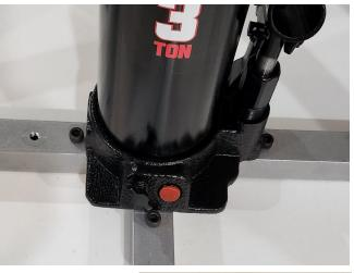
Locate the 4 clamps. Loosely assemble the clamps to the top of the braces. Slowly tighten all the bolts.
