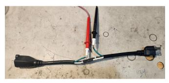
Plug the male end of the test cable into an AC source and watch the milliamps on the dvm. It may start out ok, but increase the milliamps after a half hour or so of running. You may also see evidence of oil in the water. This is an indication the seal on the pump has failed and the pump must be replaced. Around 5 milliamps will trip the gfci. <a href="https://bullerent.com/product/coolant-pump/">https://bullerent.com/product/coolant-pump/</a>
